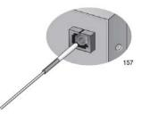
Figure 49. Cleaning a Recessed Ferrule
